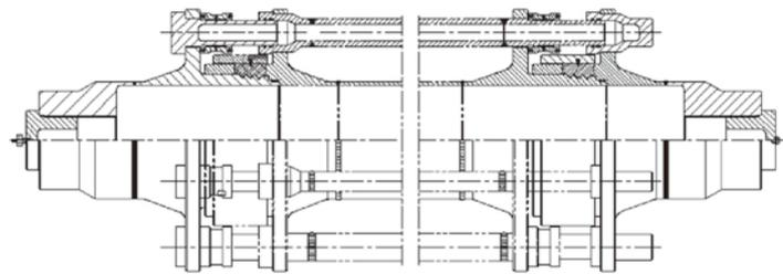
*Assembly Diagram of the Flange Type Marine Riser for Pressure Test*
